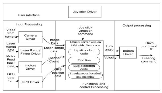
Figure 7: Software Architecture Context Diagram
