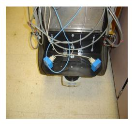
Figure 3: Ultrasonic transducers (blue boxes)
